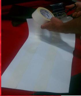
**STEP 1:** Cut a piece of the magnetized magnetic media to fit the shape of the metal parts on your printer.
