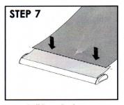
7. Peel off the adhesive cover along the edge of the base's leader roll, and attach the bottom of the banner (front facing up). Make sure the banner is straight.
