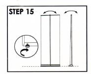
13. The unit can be levelled by adjusting the threaded feet at the bottom of the base unit.
