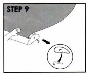
9. Remove the screw underneath the right chrome end of the base and detach. Then, with the banner held firmly, carefully pull out the retaining pin.
