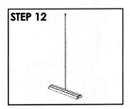
12. The bottom of the assembled pole slides into the round socket in the centre of the base unit.
