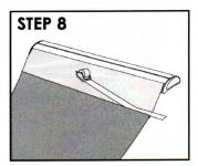
8. Finish securing the banner to the leader with a strip of wide (1 1/2" or equiv.) packing tape along the inside of the edge.
