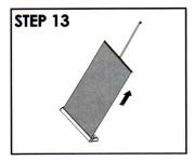
13. Unfurl the banner out of the base. (Tilting the unit backwards makes unfolding the graphic easier.)
