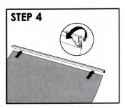
4. Swing open the beam's locking lip in order to attach the top edge of the banner. (Make sure the front of the banner is on the same side as the lip.)
