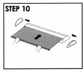
10. Carefully allow the banner to recoil into the base unit (It may be useful to have an assistant hold the base steady), then reattach the chrome end.
