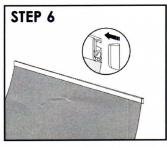
6. ...then finish the top by re-attaching the plastic end caps.
